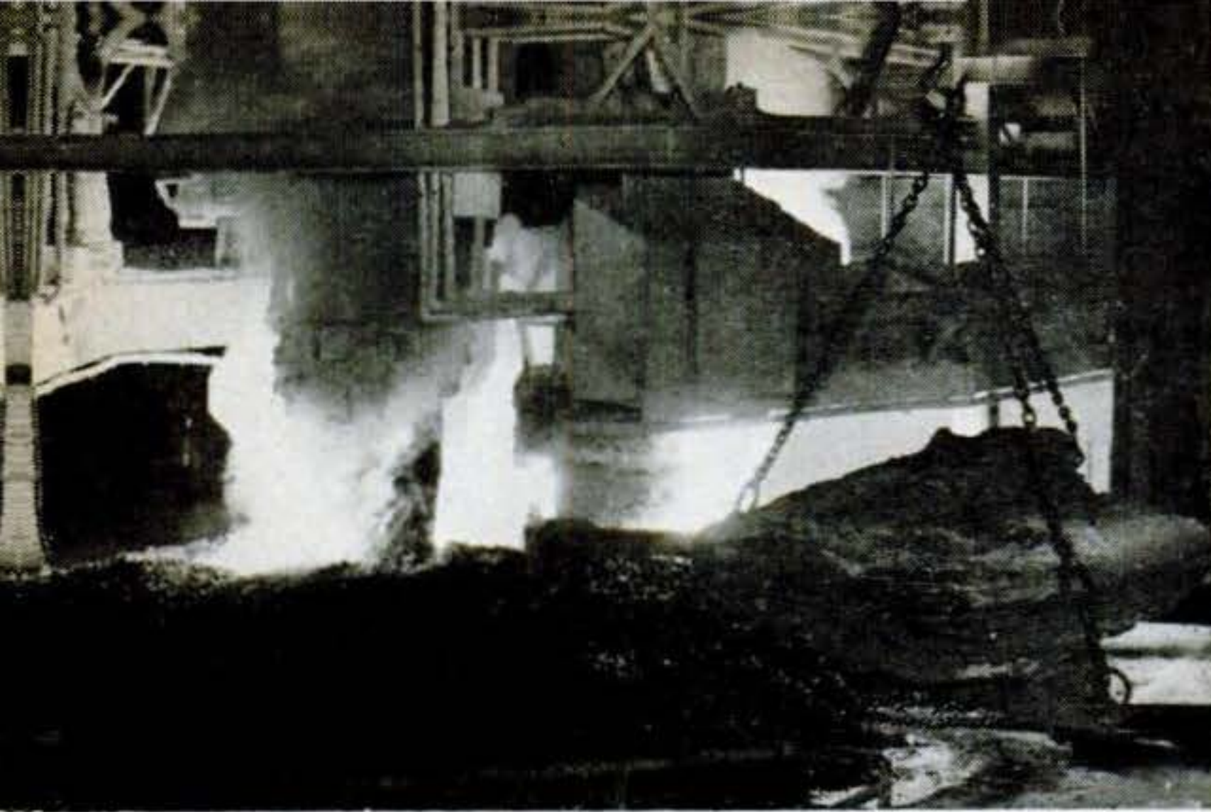
FERROSILICON , needed to smelt magnesium from dolomite, is made from quartz, coke, iron filings. At right above, ferrosilicon slabs leave furnace at Kaiser's Permanente plant.
